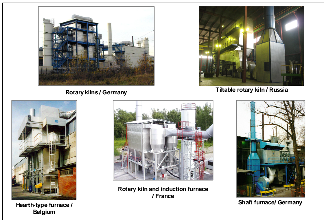
Pic. 1: Application examples for LÜHR flat-bag filters downstream melting furnaces for secondary aluminium
