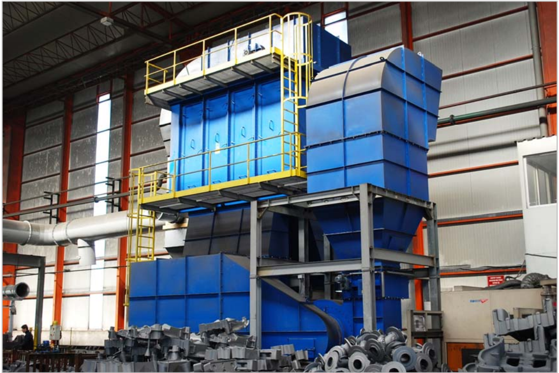
De-dusting of fettling shop
